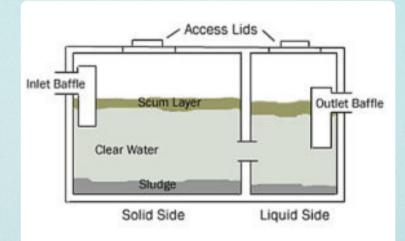
Maintaining your baffles could make the difference in spending thousands of dollars on drain field repairs, extensions, or replacements.
